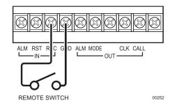
Figure 5. Connecting for Remote Recording
